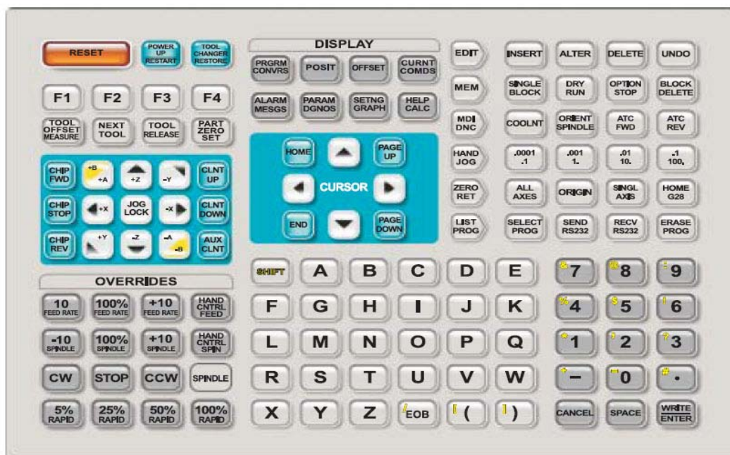
Control panel keypad with operating and display keys highlighted.
